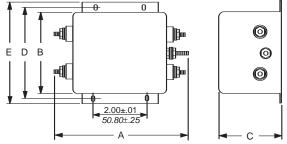
Typical dimensions: Terminals: No. 8-32 (5) Torque: 18±2 in.lb
